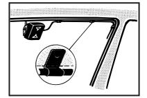
Fit matching unit by pressing it firmly into position.
