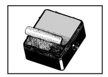
5. Remove the protective foil on the matching unit.
