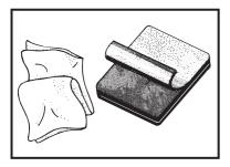
Clean both sides of the windscreen, where the antenna mount and the matching unit are to be fitted, and then remove the protective foil from the antenna mount.
